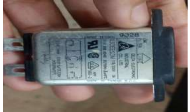
Fig. (6): Low pass filter
