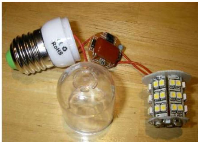
Fig. (2): LED bulb construction
