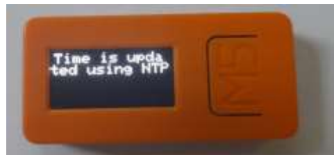
Figure (4): M5StickC LCD after time synchronization through NTP server
