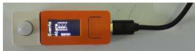
Figure (1): Solution Setup: M5StickC IoT device with PIR Hat
